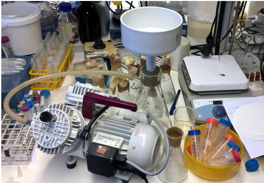
Figure 4.6: Equipment used for separating the residual solid matter after 72h of hydrolysis: Büchner flask connected to vacuum pump
